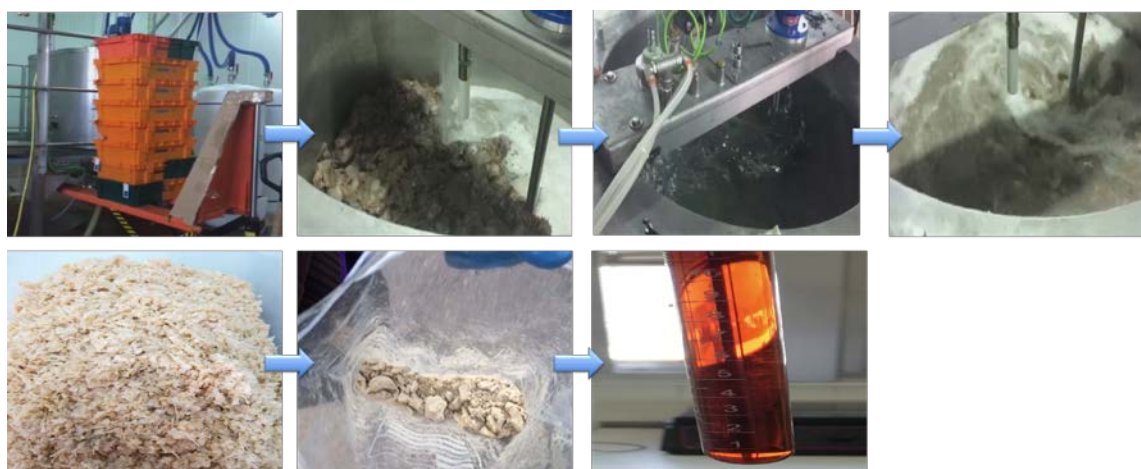
Figure 31. Steps of an enzymatic hydrolysis to produce FPHs in the iDVP3
