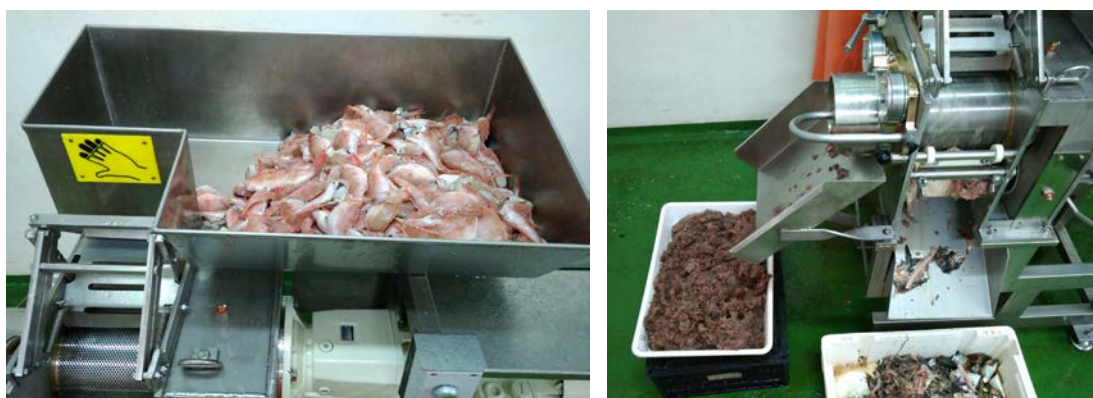
Figure 26. Developed equipment to separate fish muscle from skin and bones of different species
