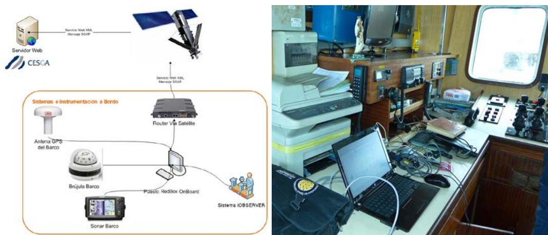
Figure 6. RedBox scheme Installation of the iObserver on-board Portosanto vessel
