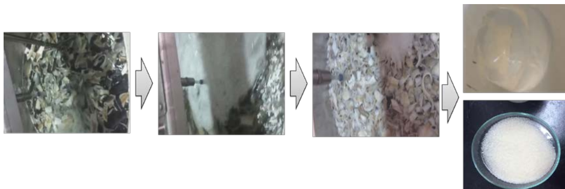
Figure 33. Gelatine obtaining from blue shark skin in the iDVP3
