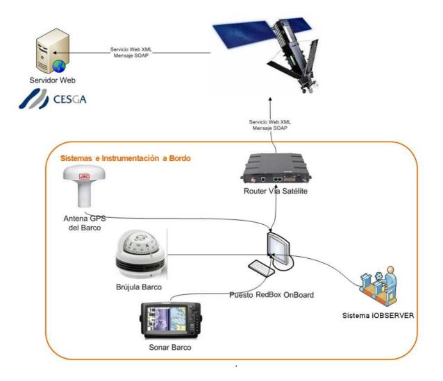
If there is a satellite router accessible for data transmission, it can also be connected to the RedBox. If there is no satellite router available, a cellular network router with WiFi connection can be used to carry out transmissions in coverage areas near the coast.
